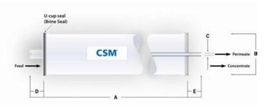
1. Each membrane elementsupplied with one brine seal, one interconnector (coupler) and four o-rings. 2. All RE2540 elementsfit nominal2.5 inch (64 mm) I.D. pressure vessels.
